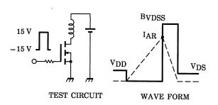
$$\begin{aligned} &R_G = 25~\Omega \\ &V_{DD} = 90~V,~L = 24.9~mH \end{aligned} \qquad EAS = \frac{1}{2} \cdot L \cdot I^2$$
